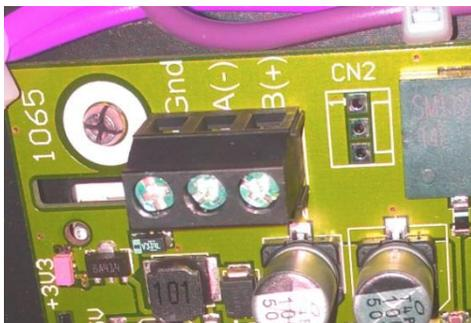
The RS-485 PORT: Both MODBUS RTU and BACNET MSTP connect to this port, selecting the protocol is done in the settings on the display. Note that the A(-) connects to D+ and B(+) connects to D-. This is very easy to get wrong.
